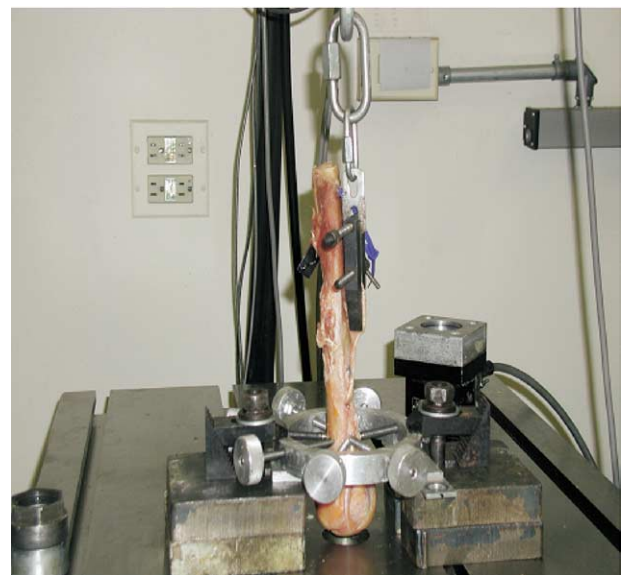
FIGURE 11. The fixture used for mounting the specimens for Instron testing. A custom-made clamp was used to couple the biceps tendon to the servohydraulic actuator. The humerus and biceps tendon were aligned such that the cyclic loading forces and ultimate pullout strength forces were parallel to the long axis of the humerus.
